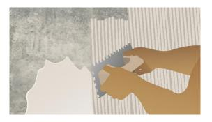
3. Apply a layer of glue cement on the wall.
