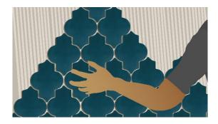
5. Place the tiles, the joint being around 3 to 4 mm and varying according to pieces since they are handcrafted, so the dimensions vary between pieces.
