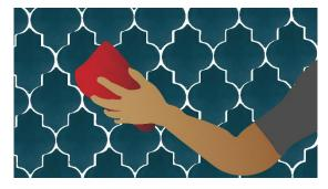
7. Finally, it must be cleaned with soap and water, removing the grouting remains with a sponge.
