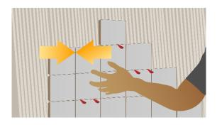
5. Place the **Zellige** tiles as close to each other, adjusting them one by one with small wedges if necessary, the joint being 1 mm sufficient.
