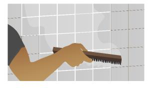
$\ensuremath{\mathsf{6}}.$  Fill joints with white or colored grouting material.
